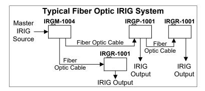
In the above diagram only two optical outputs are utilized. The IRGM-1004 provides four optical outputs.
